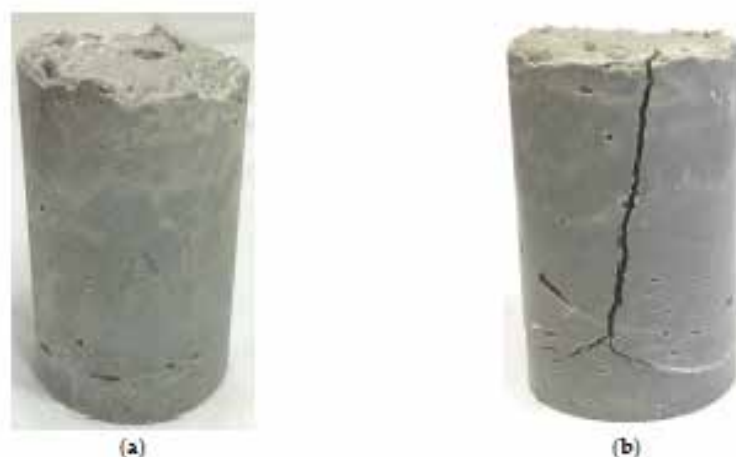
Figure 3. (a) Concrete cylinder representative for all samples and time periods except two Al containing cylinders (out of five) exposed for two years and (b) Concrete cylinder containing Al that cracked after two years of exposure.
